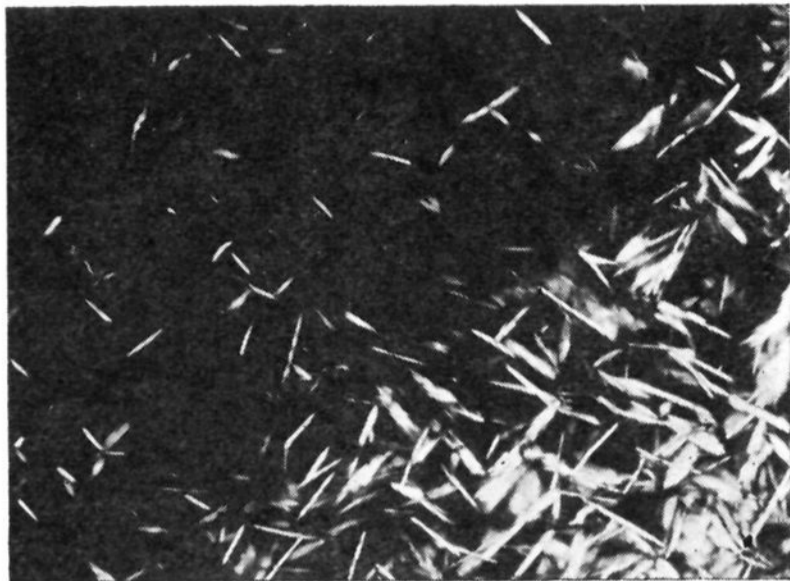
Fig. 8.—Photograph of crystals appearing below 22^\circ in distilled Fluorolube liquid (sample 2), magnification 50\times ; polarized light.
